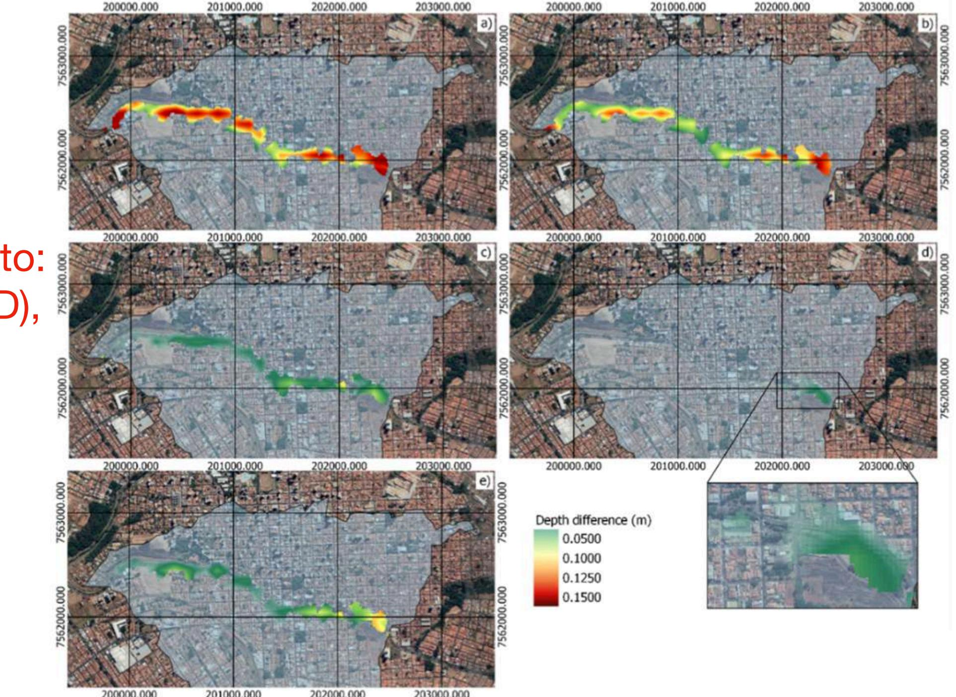
**Figure 8.** Maximum water depth difference between catchment conditions with and without LID practices for the future climate conditions. Hydrodynamic simulations with: (a) a weak rainfall input, (b) a moderate rainfall input, (c) a strong rainfall input, (d) an extreme rainfall input, and (e) the average of all rainfall inputs for the future scenario.
