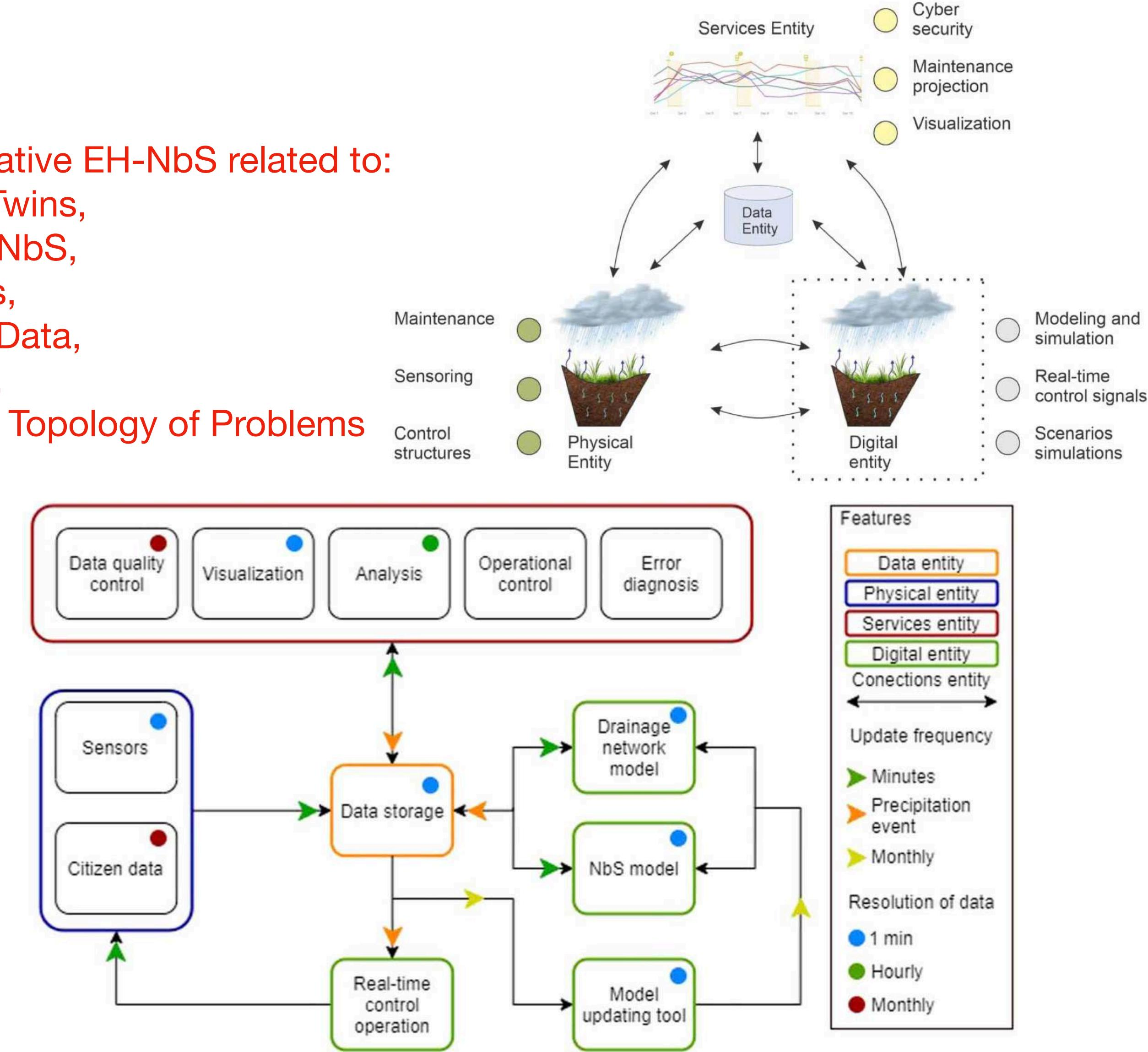
**Figure 3** | Flowchart of data flow. The data resolution and update frequency can be adapted for different NbS or different modeling techniques. Source: Adapted from Pedersen et al. (2021).
